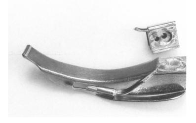
Fig. 1. Laryngoscope blade fracture between hook-on base and web
